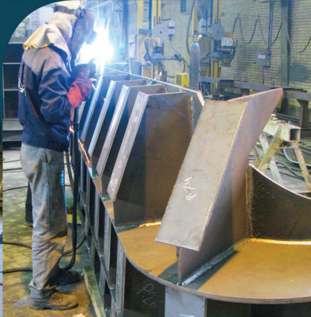
Construction and assembly of super-structure boilers of Jajarm aluminum ingots
