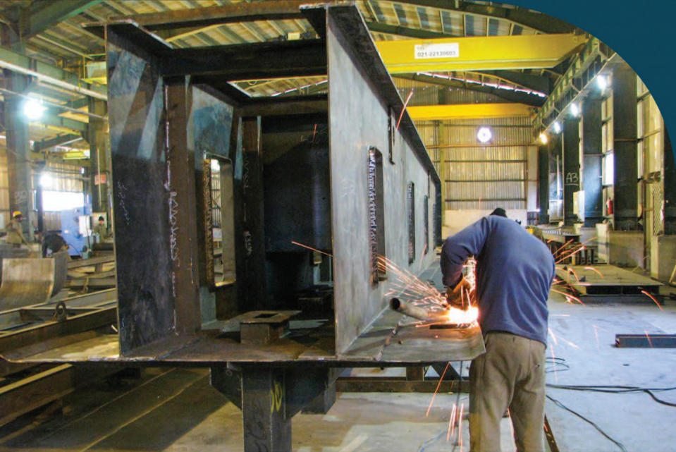
Construction and assembly of super-structure boilers of Jajarm aluminum ingots
